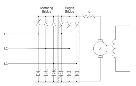
The motor receives power from the incoming line. In this example the motor is operating at full speed (500 VDC).
