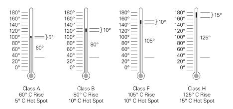
The operating temperature of a motor is important to efficient operation and long life. Operating a motor above the limits of the insulation class reduces the motor's life expectancy. A 10°C increase in the operating temperature can decrease the life expectancy of a motor by as much as 50%. In addition, excess heat increases brush wear.
