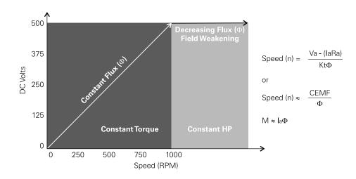
Horsepower is said to be constant because speed (N) increases and torque (M) decreases in proportion.
