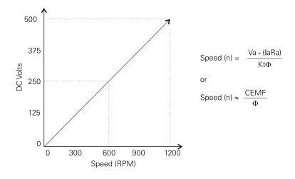
The base speed listed on a motor's nameplate, however, is an indication of how fast the motor will turn with rated armature voltage and rated load (amps) at rated flux ( $\Phi$ ).
