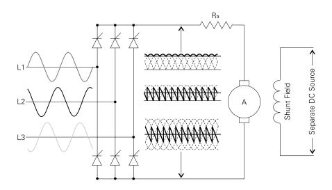
It is important to note that the voltage applied to a DC motor be no greater than the rated nameplate. Armature windings are commonly wound for 500 VDC. The control logic in the drive must be adjusted to limit available DC voltage to 0 - 500 VDC. Likewise, the shunt field must be limited to the motor's nameplate value.
